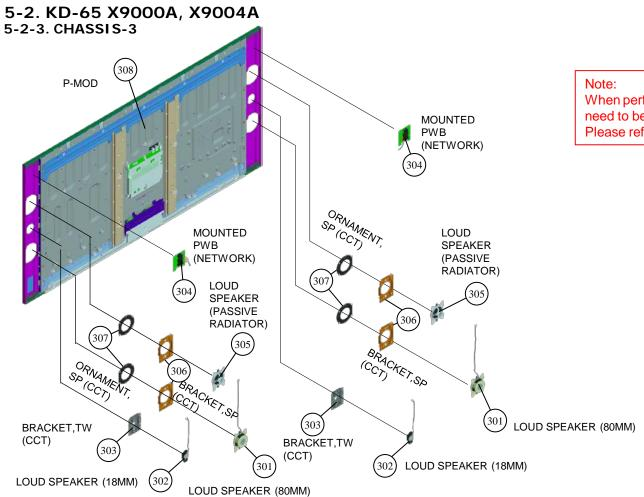
When performing panel replacement, these synchronize and need to be replaced to new parts.
