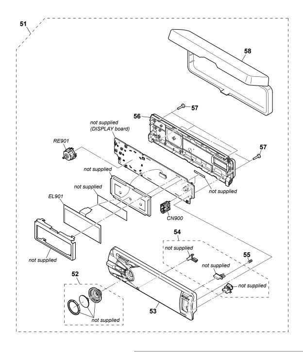
**Note:** Refer to the servicing notes "NOTE FOR REPLACEMENT OF THE USB CONNECTOR (CN900)" (See page 5), if replacing the Ref. No. CN900.
