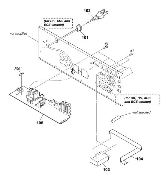
**Note:** If wire (flat type) is replaced, install it after bending it in the same form as that before replacement.
