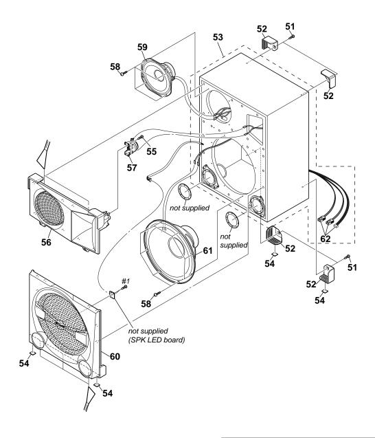
**Note:** This diagram is for L channel speaker. The mechanical position of R channel is reversed.
