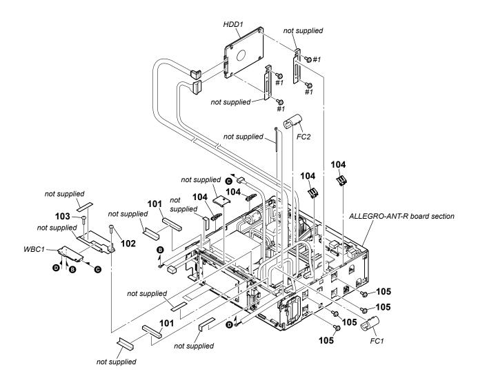
Note 1: When the WLAN/BT COMBO card (Ref. No. WBC1) is replaced, refer to "NOTE OF REPLACING THE WLAN/BT COMBO CARD AND CHECKING METHOD OF NETWORK CONNECTION" on page 5.
