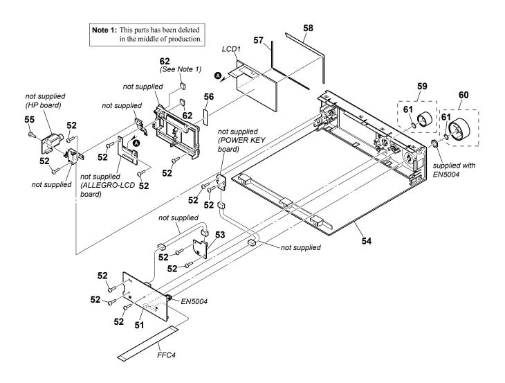
**Note 2:** Wires (flat type) for service is straight. When replacing wire (flat type), install it after bending it in the same form as that before replacement.
