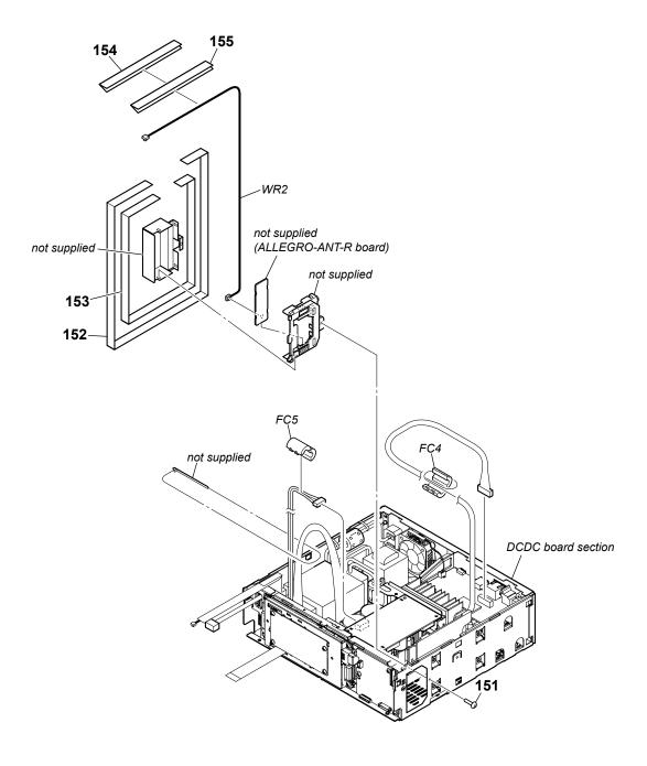
**Note:** When the coaxial (U.FL connector) cable (Ref. No. WR2) is replaced, refer to "NOTE OF REPLACING THE WLAN/BT COMBO CARD AND CHECKING METHOD OF NETWORK CONNECTION" on page 5.
