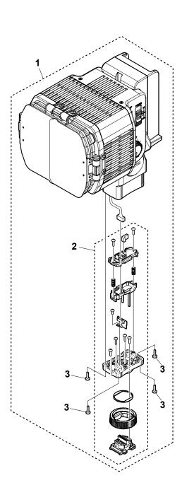
Note 1: The repair part for the SHOE HOLDER (S) ASSY (Ref. No. 2) comes assembled as shown in the figure below. When installing the SHOE HOLDER (S) ASSY to the UNIT, do so after disassembly.
