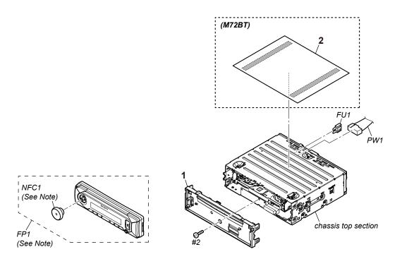
Note: When replacing the panel front assy (Ref. No. FP1) or knob (VOL) assy (Ref. No. NFC1), make sure to refer to "NOTE OF REPLAC-ING THE PANEL FRONT ASSY OR THE KNOB (VOL) ASSY" on page 6.
