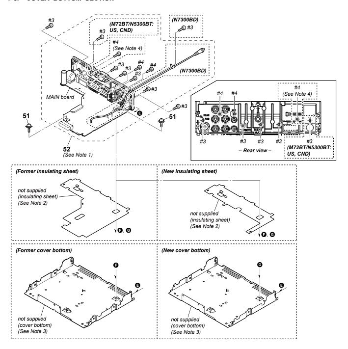
**Note 1:** When the complete MAIN board (Ref. No. 52) is replaced, be sure to replace the knob (VOL) assy (Ref. No. NFC1: page 65) simultaneously. Also, be sure to referring to "NOTE OF REPLACING THE MAIN BOARD" on page 6.
